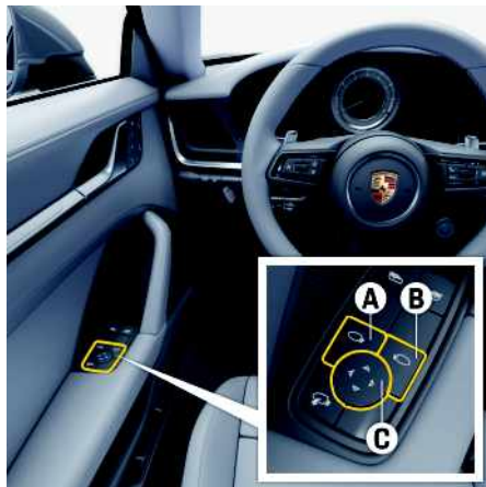
Fig. 130: Swivelling down mirror glass as parking aid
