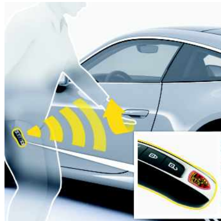
Fig. 30: Unlocking door with Comfort Access
