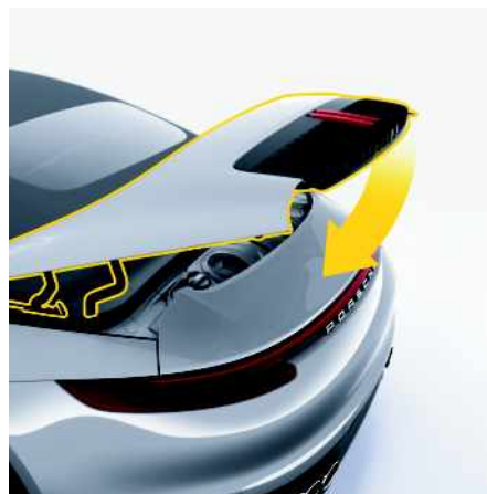
Fig. 66: Closing the convertible-top compartment lid
