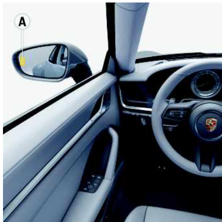
Fig. 98: Warning indicator A on the exterior mirror
