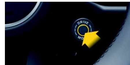
Fig. 79: SPORT Response button on the steering wheel
