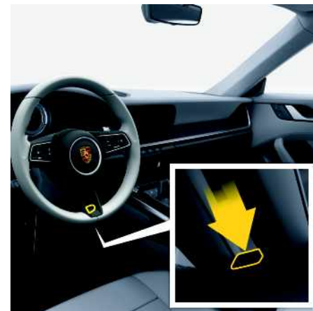
Fig. 192: Heated steering wheel button
