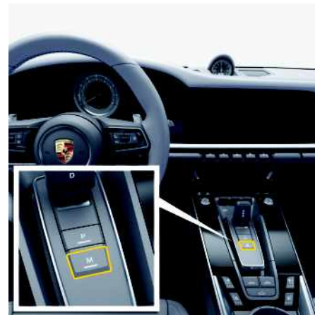
Fig. 208: Manual shifting mode
