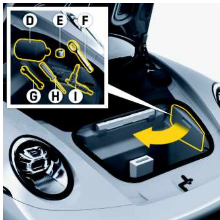
Fig. 114: Tyre sealing compound and tool kit
