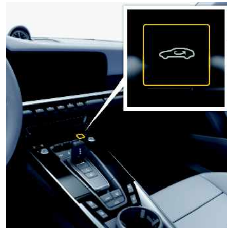
Fig. 18: Switching air-recirculation mode on and off
