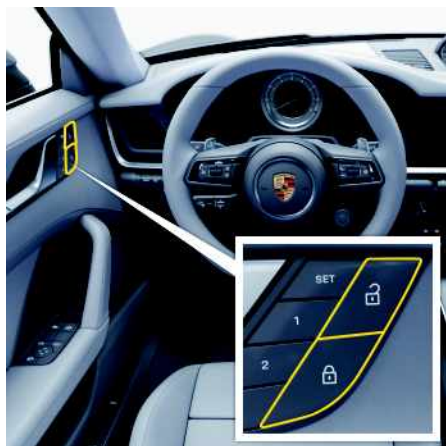
Fig. 31: Central locking button in the door panel
