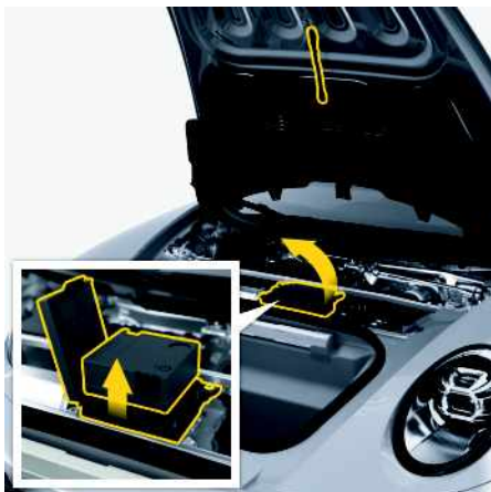
Fig. 117: Opening storage compartment for tyre filling compressor
