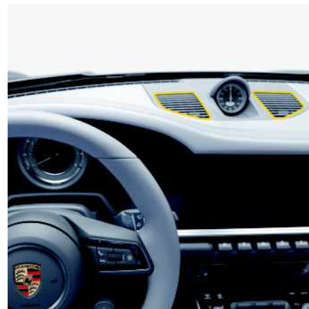
Fig. 17: Adjusting the upper ventilation panel
