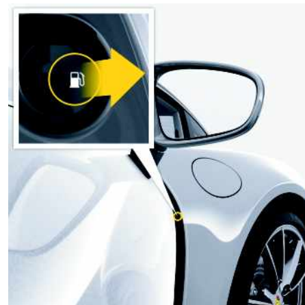
Fig. 159: Emergency operation of the filler flap
