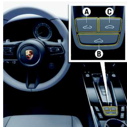
Fig. 179: Operating steel slide/tilt roof
