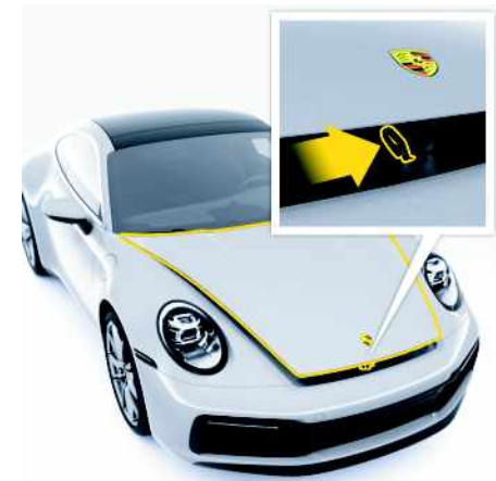
Fig. 121: Unlocking luggage compartment lid
