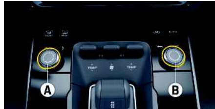
Fig. 144: Volume control and rotary push button
