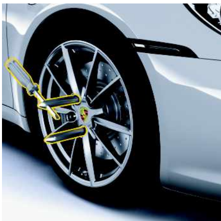
Fig. 219: Screw in two assembly aids on vehicles with PCCB
