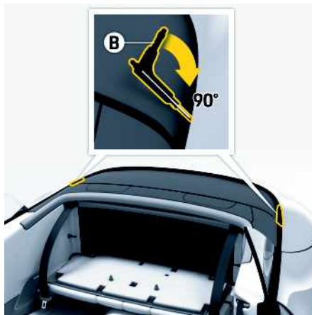
Fig. 56: Unlocking the convertible-top compartment lid (step 1)
