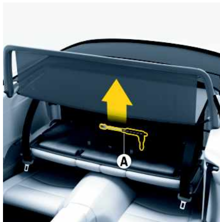
Fig. 49: Removing the emergency operation key
