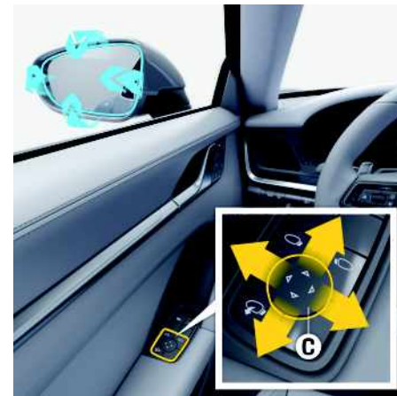
Fig. 128: Adjusting exterior mirrors
