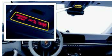
Fig. 40: PASSENGER AIR BAG OFF/ON indicator
