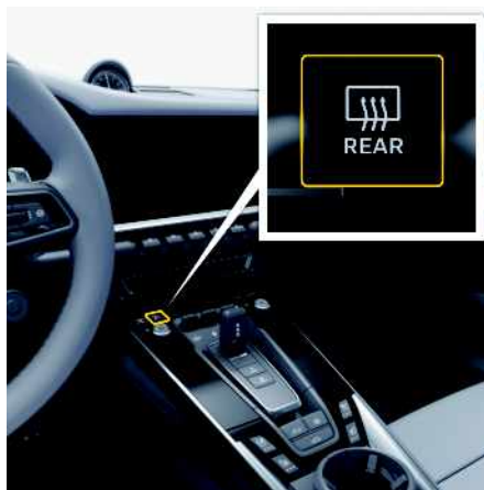
Fig. 20: Heated rear window/exterior mirror heating button
