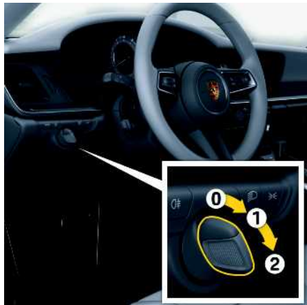
Fig. 189: Ignition lock positions
