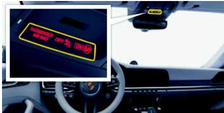
Fig. 8: PASSENGER AIR BAG OFF/ON indicator
