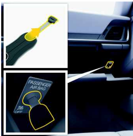
Fig. 39: Switching off the passenger airbag
