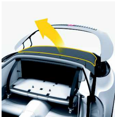
Fig. 62: Pulling convertible top out of storage compartment
