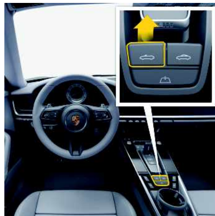
Fig. 45: Opening the convertible top with the button
