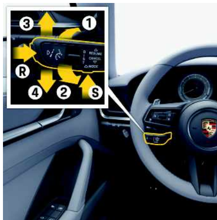
Fig. 68: Control stalk for driver assistance systems
