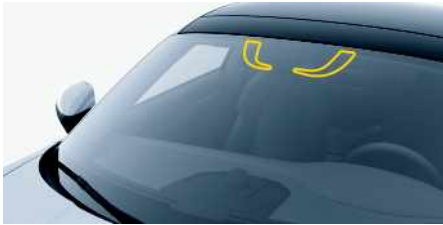
Fig. 135: Attaching toll devices
