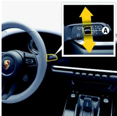
Fig. 226: Switch for rain sensor/intermittent operation
