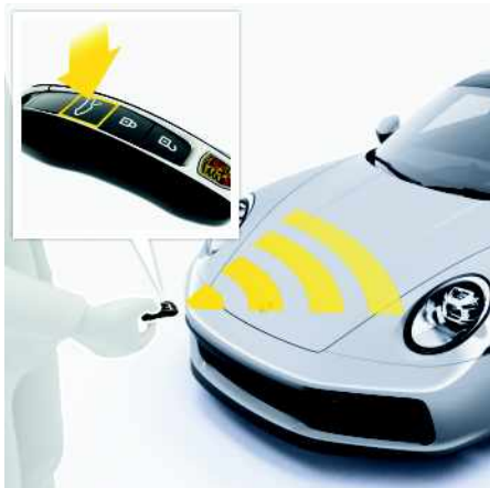
Fig. 122: Opening luggage compartment lid with driver's key
