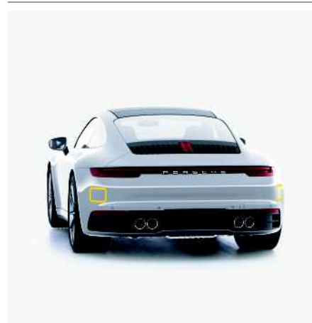
Fig. 99: Radar sensors in the rear bumper
