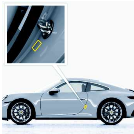
Fig. 230: Tyre pressure plate fixing point
