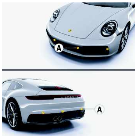
Fig. 139: Sensors for distance measurement
