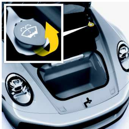
Fig. 170: Washer fluid reservoir for windscreen
