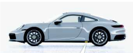
Fig. 94: Front jacking point for jack and lifting platform
