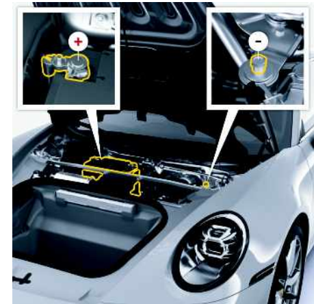
Fig. 22: Lead battery terminals
