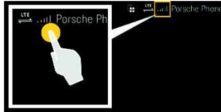
Fig. 12: Opening the Device Manager
