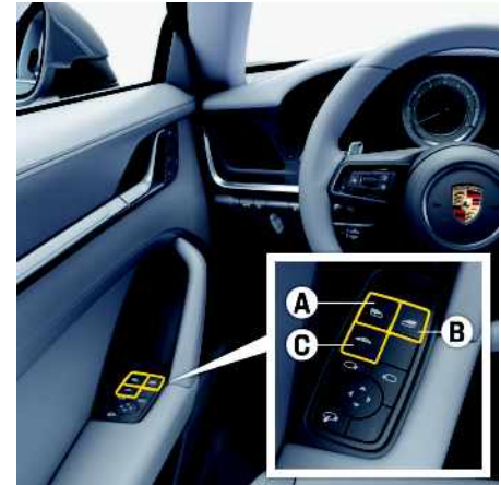
Fig. 221: Power window buttons in driver's door
