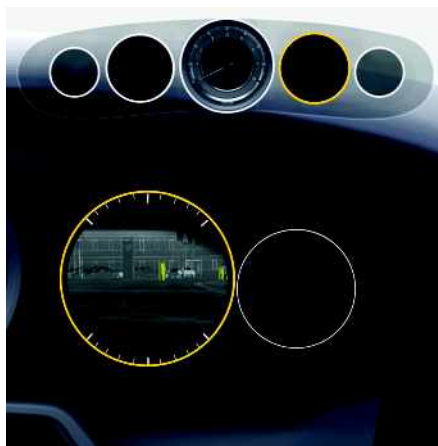
Fig. 136: Night View Assist thermal image
