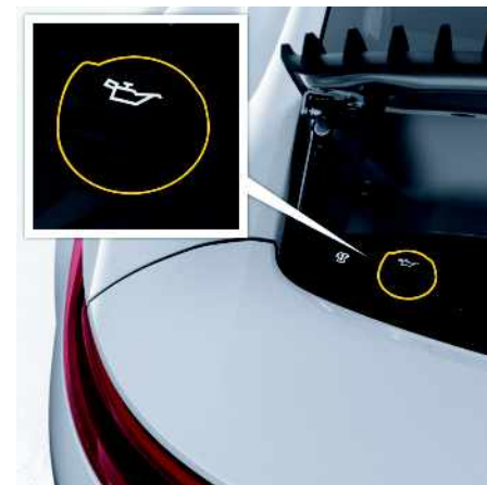
Fig. 86: Oil filler opening
