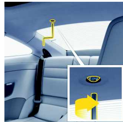
Fig. 182: Closing the slide/tilt roof with the hexagon key
