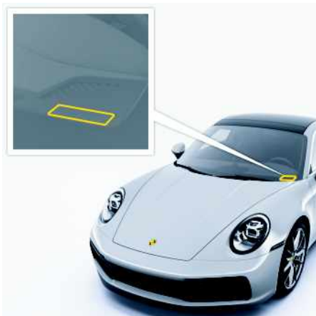
Fig. 228: Vehicle identification number fixing point
