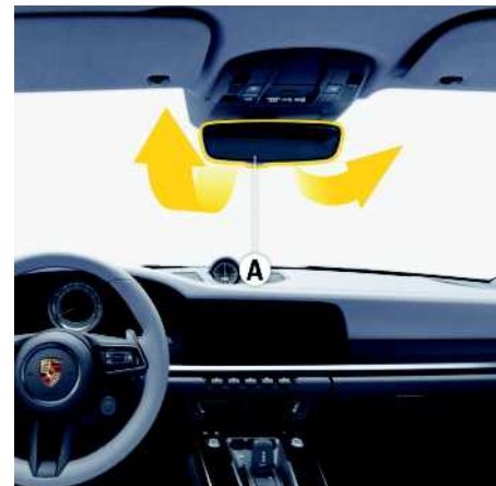
Fig. 131: Dimming interior mirror manually
