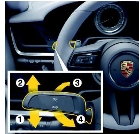
Fig. 111: Operating direction indicators, high beam and headlight flasher
