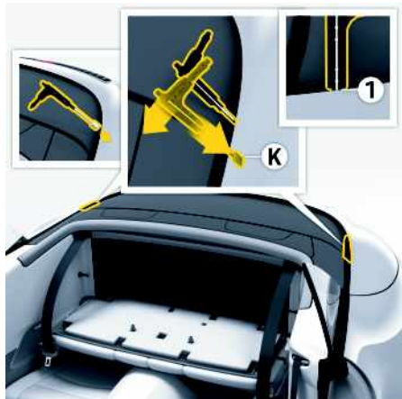
Fig. 55: Insert the emergency operation key.
