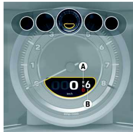
Fig. 206: Indicator for operating mode and engaged gear
