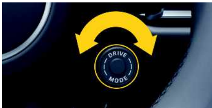
Fig. 77: Driving programme at the steering wheel
