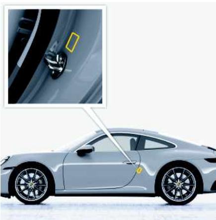
Fig. 229: Identification plate fixing point
