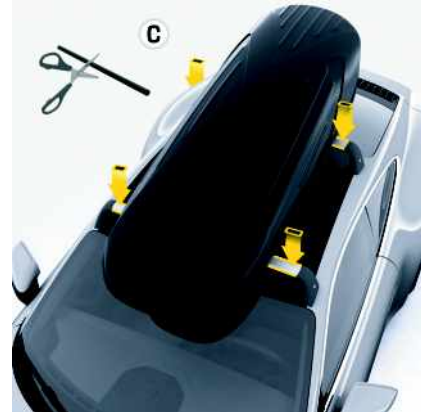
Fig. 169: Cutting the cover trims to size and attaching
