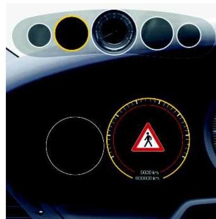
Fig. 137: Pedestrian warning on the instrument cluster.
