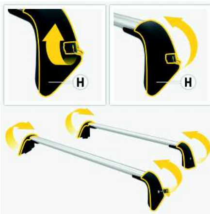
Fig. 163: Unlocking and folding up the cover flaps
