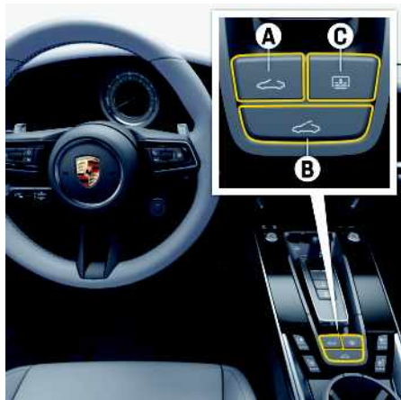
Fig. 180: Operating the glass slide/tilt roof
