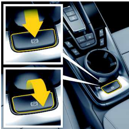
Fig. 26: Electric parking brake button
