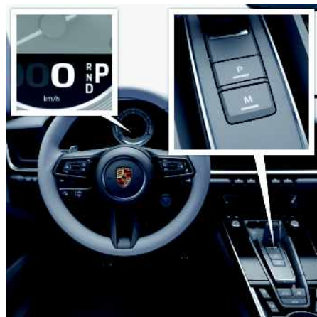
Fig. 207: Engaging the parking lock
