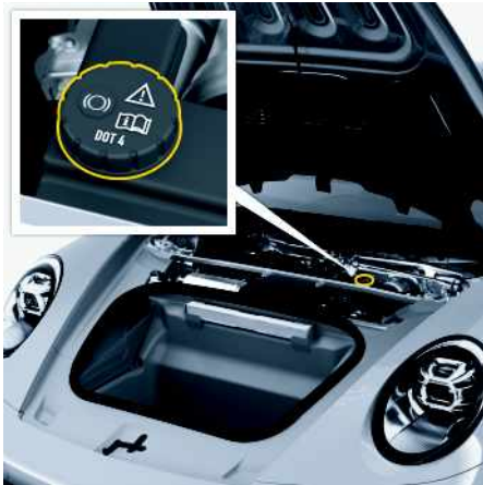
Fig. 25: Brake fluid reservoir
