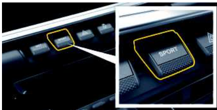
Fig. 76: Buttons for driving programme (e.g. SPORT)
