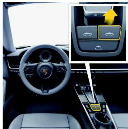
Fig. 46: Closing the convertible top with the button
