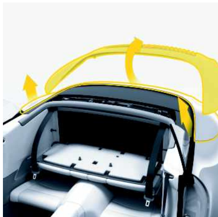
Fig. 58: Raising the convertible-top compartment lid
