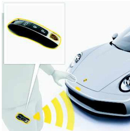
Fig. 123: Opening luggage compartment lid with Comfort Access
