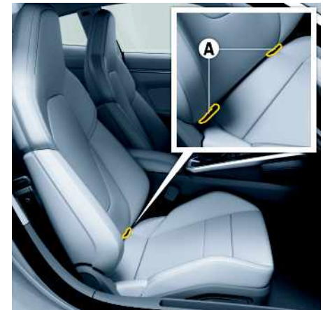
Fig. 41: ISOFIX anchorage system on passenger seat
