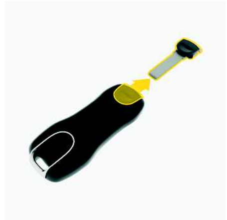
Fig. 74: Removing emergency key
