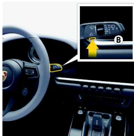
Fig. 138: Button for camera washer system
