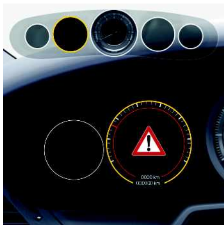
Fig. 142: Collision warning on the instrument cluster
