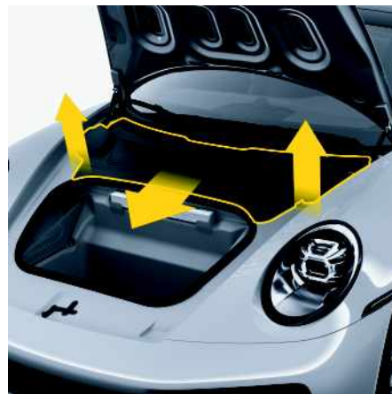
Fig. 115: Detaching and lifting plastic cover
