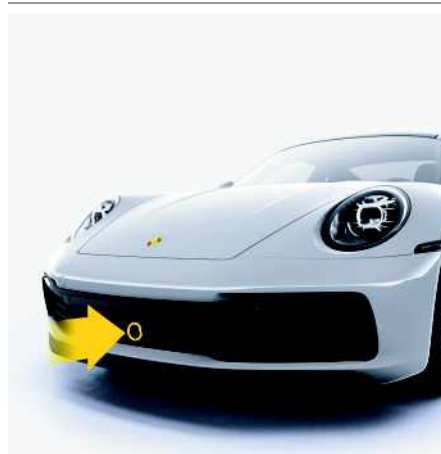
Fig. 1: Location of radar sensor
