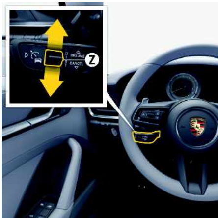
Fig. 7: Setting the desired distance
