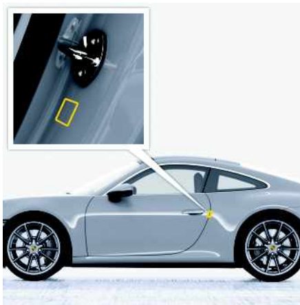
Fig. 213: Tyre pressure plate
