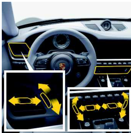
Fig. 16: Adjusting air vents
